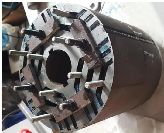
*Fig. 5.4 photograph of the PVC filling inside of the rotor flux barriers*
