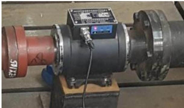
Fig. 5.13 Torque transducer coupled with the shaft
