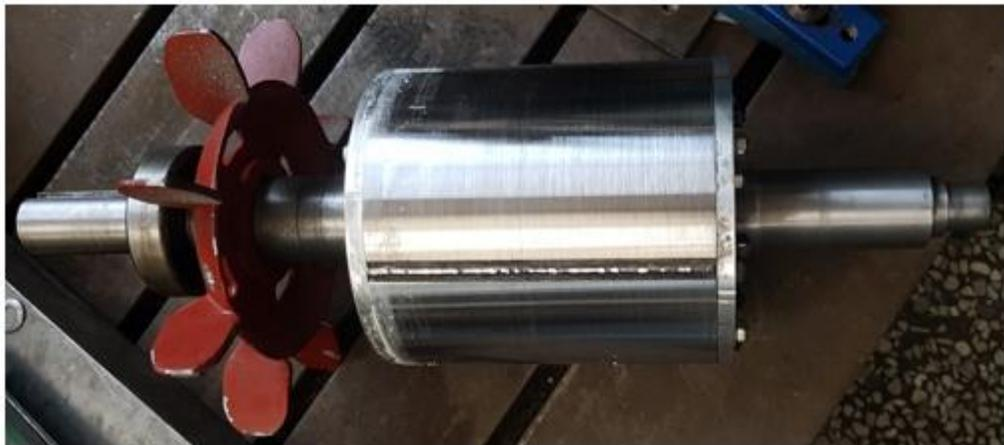
*Fig. 5.7 photograph of the assembled rotor after machining*
