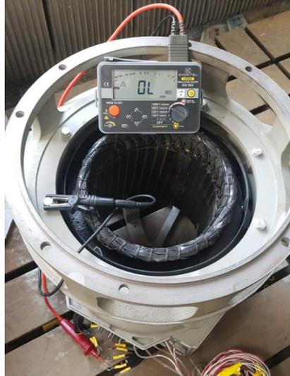
*Fig. 5.16 photograph of 3-phase stator winding megger testing*
