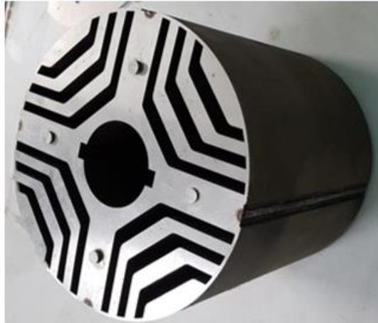
*Fig. 5.3 photograph of the manufactured rotor from the factory*
