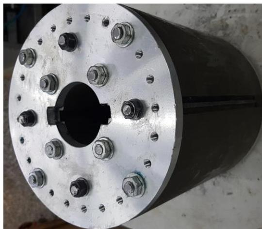
*Fig. 5.5 photograph of the PVC filling inside of the rotor with cover plate*
