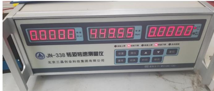
Fig. 5.12 Torque measuring instrument JN-338 series
