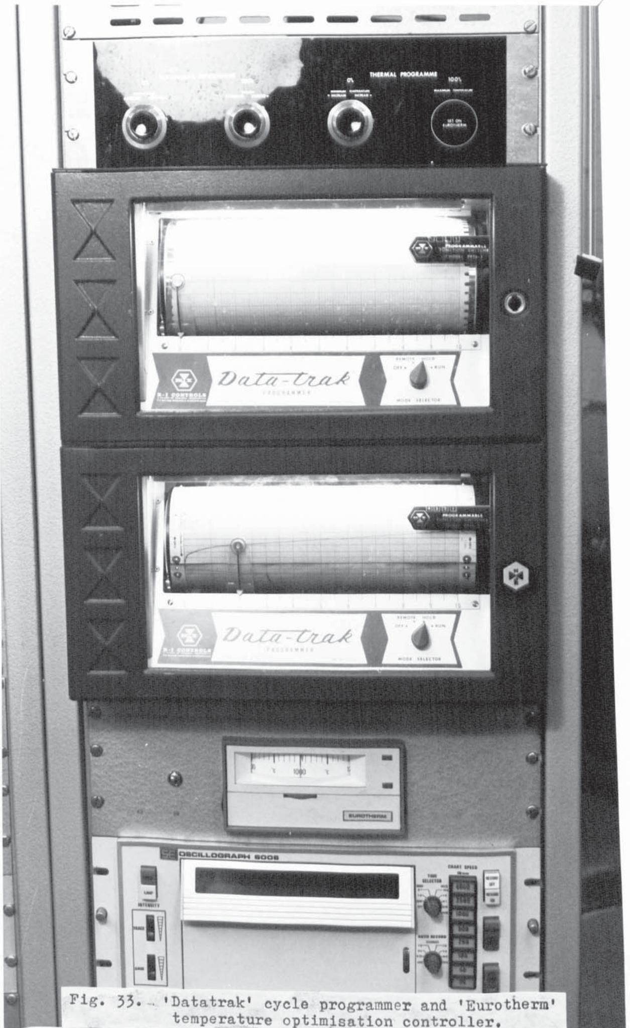
Fig. 33. 'Datatrak' cycle programmer and 'Eurotherm' temperature optimisation controller.
