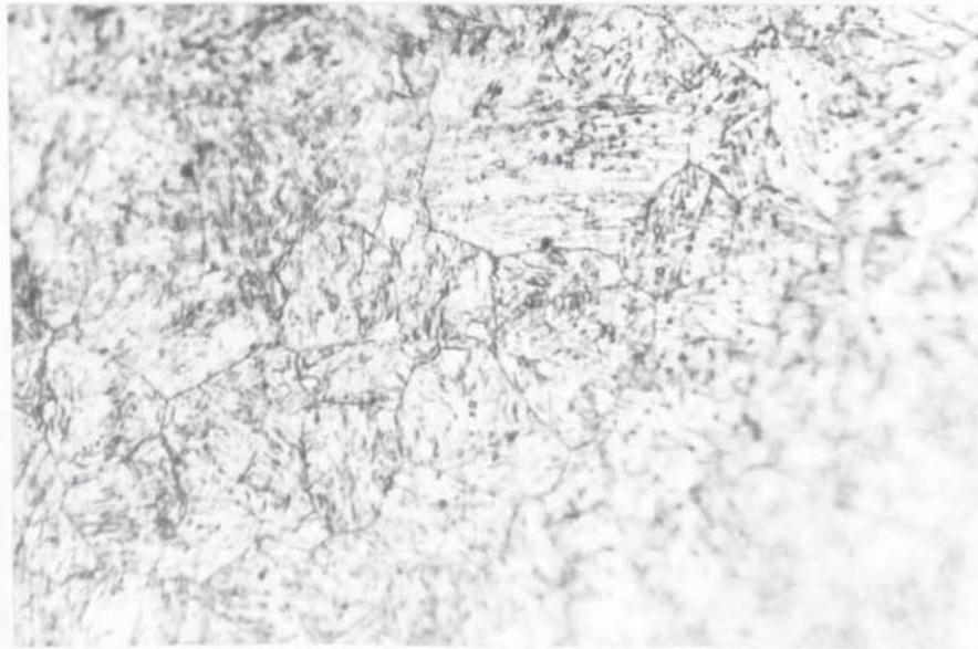
(b) Welded. Electrolytic polish/etch. X 1400
