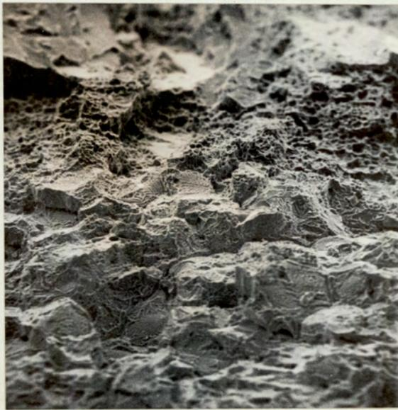
Fig.28. Weld Specimen EC showing Intergranular H.A.Z. region with no hot cracks and Grain Faces completely covered with Fern Dendrites and Ductile Dimpling.
