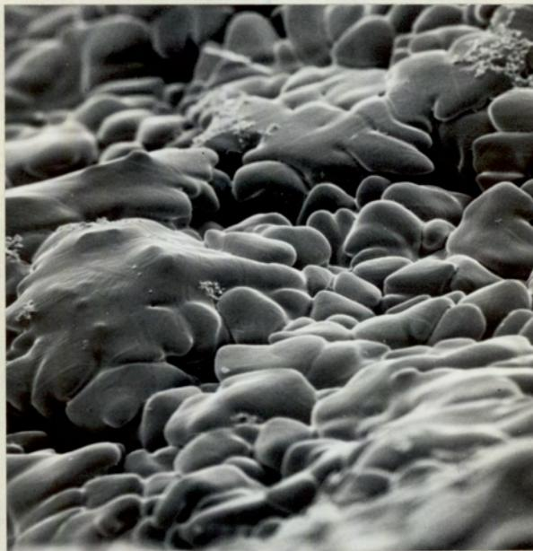
Fig.63. Fracture Face of SAE 4130, SC, Hot Ductility Specimen, broken on heating at 1510° C, (within 6° C of the Bulk Melting Temperature), showing Extensive Rounding of Grains.
