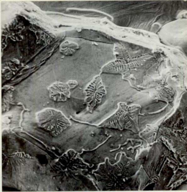
Fig.24. Weld Specimen, SD, showing Fern Dendrites standing proud of Crack Surface.
