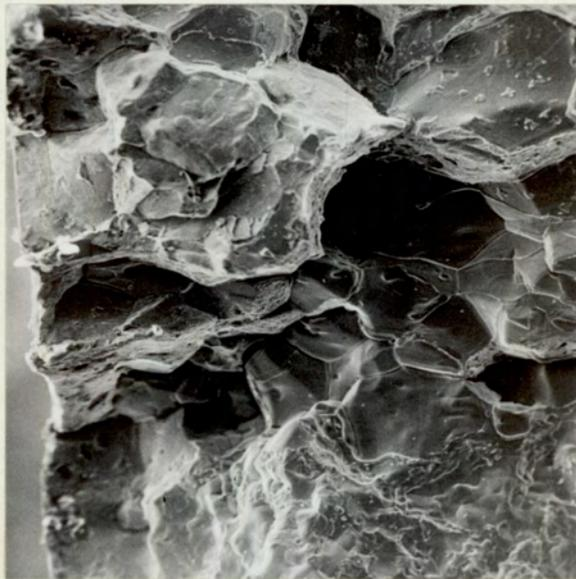
Fig.17. Crack Sensitive SD Weld Specimen, showing detail of Weld Metal Intergranular H.A.Z. Boundary.
