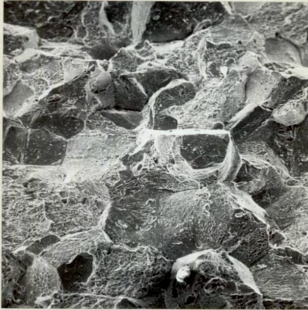
Fig. 78. Fracture Face of SAE 4130, SA, Hot Ductility Specimen, Thermally Cycled to 1496° C, and Impact Tested at 100° C, showing Intergranular Failure.
