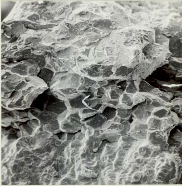
Fig.16. Crack Sensitive SD Weld Specimen showing 3 zones in Weldment, namely, Weld Metal, Intergranular H.A.Z., and Transgranular H.A.Z.
