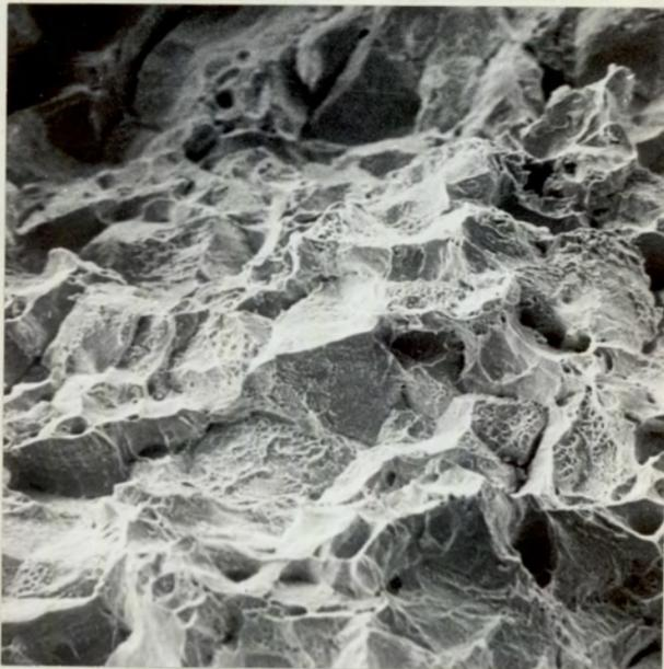
Fig. 71. Fracture Face of SAE 4130, SC, Hot Ductility Specimen, broken on Cooling at 930° C, with 40% R.A., from a Peak of 1480° C, showing Partial Return to Intergranular Failure.
