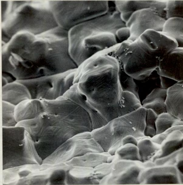
Fig.62. Fracture Face of SAE 4130, SC, Hot Ductility Specimen, broken on heating at 1488° C, with 0% R.A., showing Intergranular Failure with a more rounded Profile.
