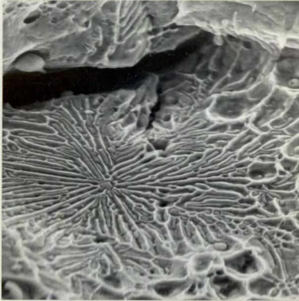
Fig.80. Fracture Face of SAE 4130, SA, Hot Ductility Specimen, Thermally cycled to 1496° C, and Impact Tested at 100° C, showing detail of Fern Dendrite.
