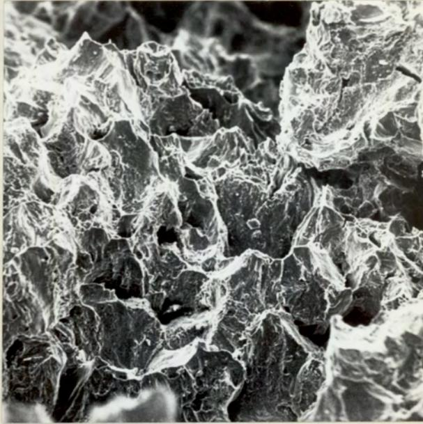
Fig. 70. Fracture Face of SAE 4130, SC, Hot Ductility Specimen, broken on Cooling at 1240° C, with 32% R.A., from a Peak of 1477° C, with 32% R.A., showing a predominantly Ductile Failure Mode.
