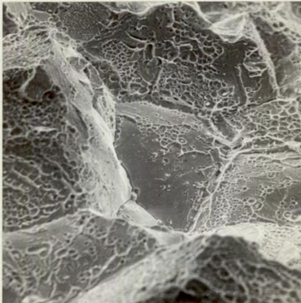
Fig.81. Fracture Face of SAE 4130, SA, Hot Ductility Specimen, Thermally cycled to 1496° C, and Impact Tested at 100° C, showing detail of Ductile Dimples at the Grain Faces.
