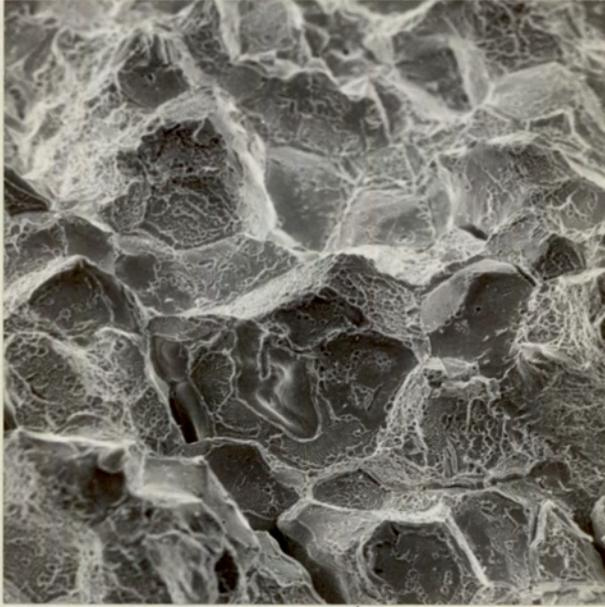
Fig.82. Fracture Face of SAE 4130, SA, Hot Ductility Specimen, Thermally Cycled to 1496° C and Impact Tested at 100° C, showing Free Surface Areas and Associated Fern Dendrites.
