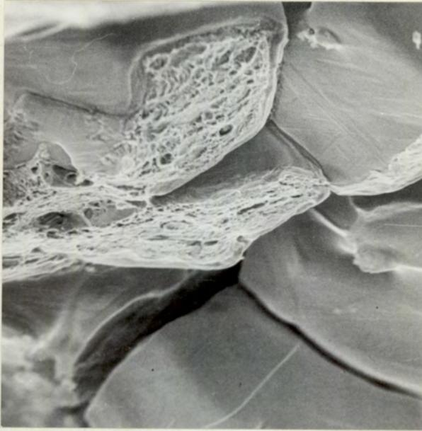
Fig.22. Crack Sensitive SD Weld Specimen showing Branching Cracks
