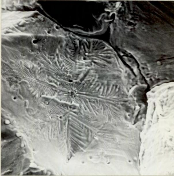
Fig. 76. Fracture Face of SAE 4130<sub>0</sub> SC, Hot Ductility Specimen, broken on Cooling at 1324° C, with 0% R.A., after Peak of 1506° C. showing Fern Dendrite at Grain Boundary.
