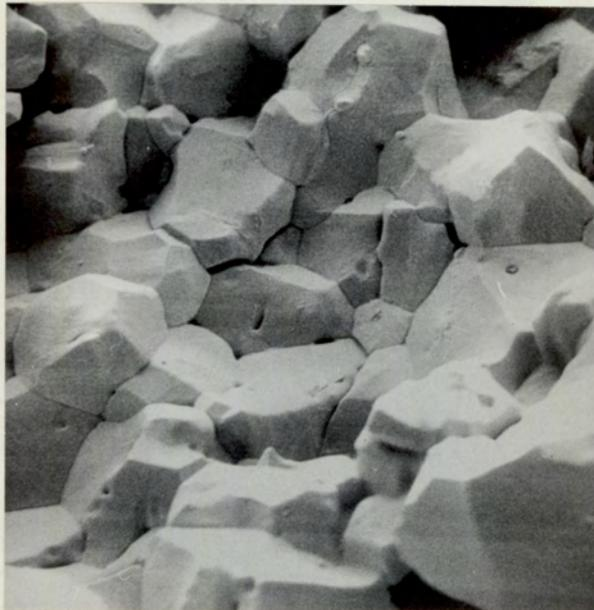
Fig.60. Fracture Face of SAE 4130<sub>6</sub> SC, Hot Ductility Specimen, broken on heating at 1446 C, with 0% R.A., showing Intergranular Failure. (Note holes at grain faces).
