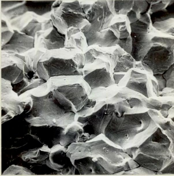
Fig. 74. Fracture Face of SAE 4130, SC, Hot Ductility Specimen, broken on Cooling at 1368° C, with 0% R.A., after Peak of 1504° C, showing more Angular Grain outline.
