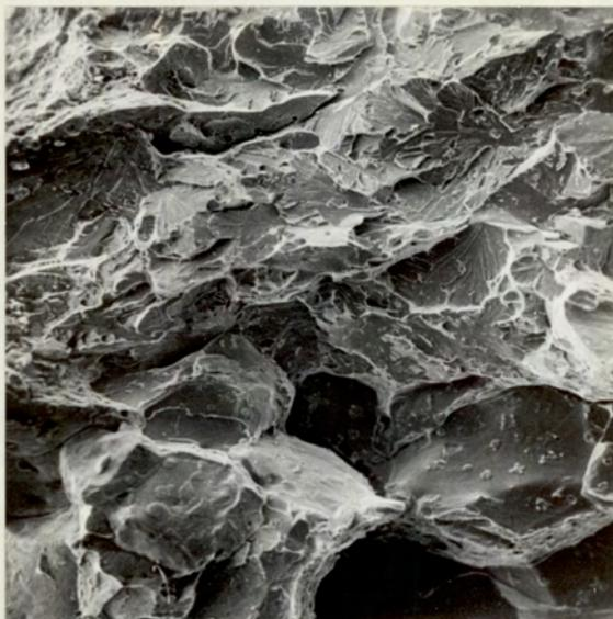
Fig.18. Crack Sensitive SD Weld Specimen showing detail of Intergranular - Transgranular H.A.Z. Boundary.
