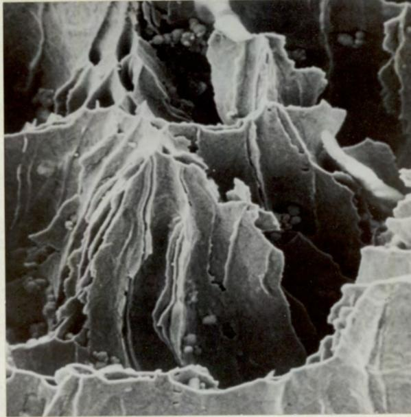
Fig.59. Fracture Face of SAE 4130<sub>6</sub> SA, Hot Ductility Specimen broken on heating at 1380 C, with 98% R.A., showing Ductile Failure.
