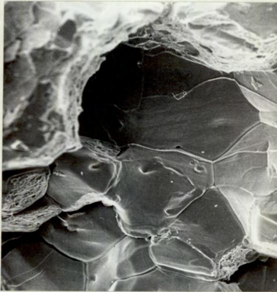
Fig.23. Crack Sensitive SD Weld Specimen, showing Holes
