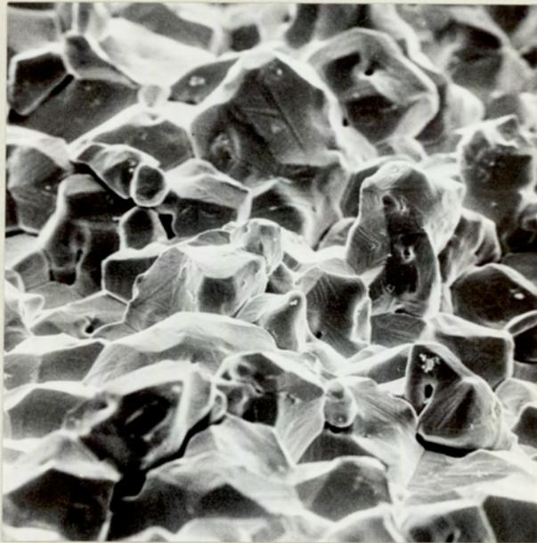
Fig.66. Fracture Face of SAE 4130, SC, Hot Ductility Specimen, broken on Cooling at 1432° C, with 0% R.A., after Peak of 1480° C, showing Sharper Intergranular Profile.
