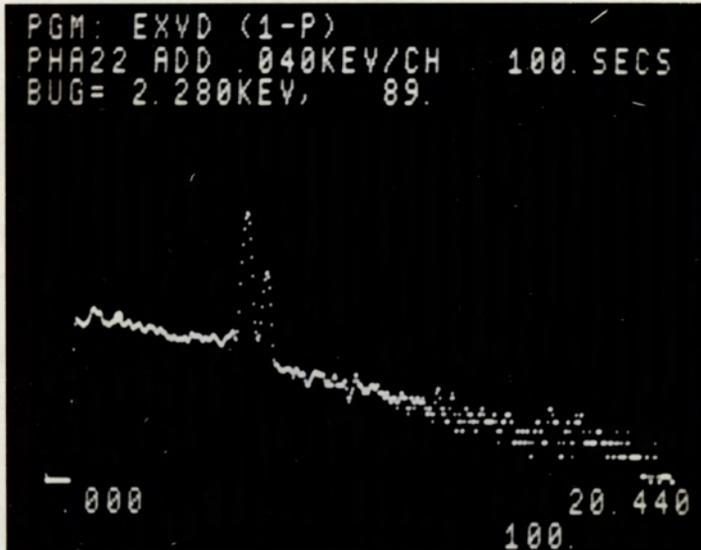
Fig.27. Energy Spectrum from Hot Crack Surface in Steel, SC.
