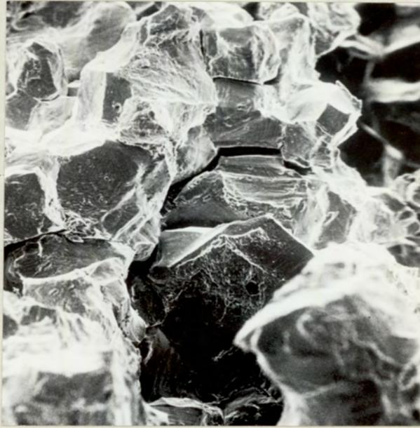
Fig.68. Fracture Face of SAE 4130, SC, Hot Ductility Specimen, broken on Cooling, at  $1376^{\circ}\text{C}$ , with 6% R.A., after peak of  $1473^{\circ}\text{C}$ , showing large Areas of Ductile Dimpling at Grain Faces.
