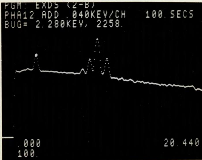
Fig.26. Energy Spectrum from Rod Inclusion in Steel, SC.
