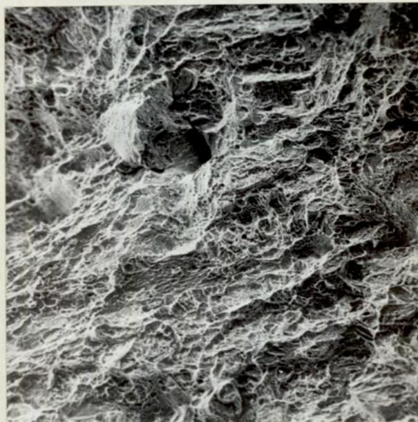
Fig. 79. Fracture Face of SAE 4130, SA, Hot Ductility Specimen, Thermally Cycled above the Melting Temperature of 1516° C, and Impact Tested at 100° C, showing no Intergranular Zone.
