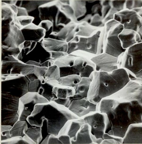
Fig.61. Fracture Face of SAE 4130, SC, Hot Ductility Specimen, broken on heating at 1474° C, with 0% R.A., showing Intergranular Failure.
