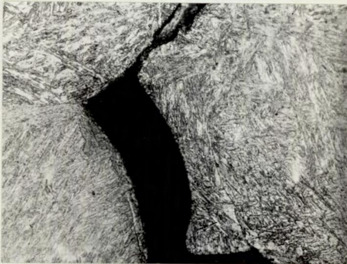
Fig.11. High Temperature Intergranular Cracking in the Weld Heat Affected Zone of SAE 4130.
