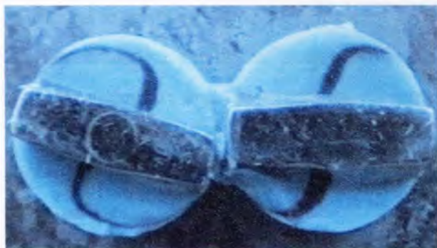
Figure 8-4 A slice through a two coloured clay mixture revealing the deformation of a horizontal plane after a 1/2\pi rotation of the left rotor
