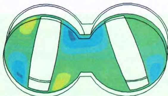
Figure 7-17 'Z' velocity contours for n=0.4
