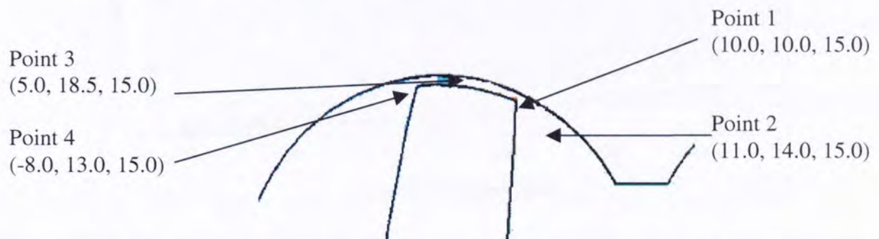
Figure 7-28 Probe location for viscoelastic extra stress investigation on rotor configuration 2
