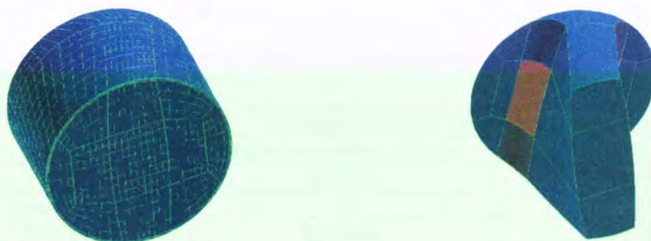
Figure 8-1a) Left/right rotor fluid domain. b) Left/right rotor wall boundary on its own.
