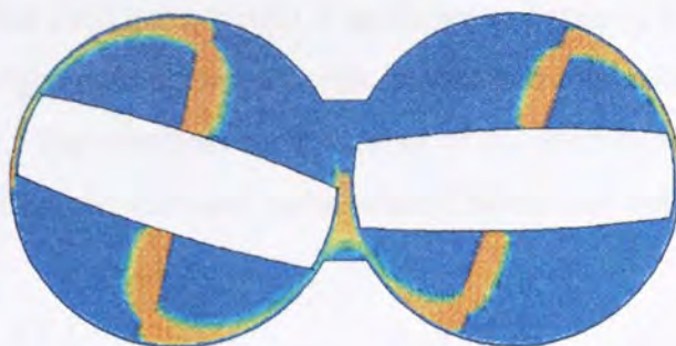
Figure 8-4 A slice through a two coloured clay mixture revealing the deformation of a horizontal plane after a 1/2\pi rotation of the left rotor
